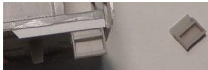
8. Below is the smoke stack which is needed to be short. Here we have modified the smoke stack and made it shorter. They were glued back together with Plastruct Bondene Solvent Cement.
