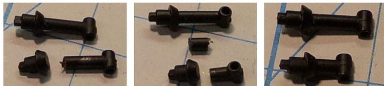
9. Now we need to drill a hole in the roof for the smoke stack. The smoke stack base is 2.33 mm. After drilling the hole, we test fit the smoke stack.
