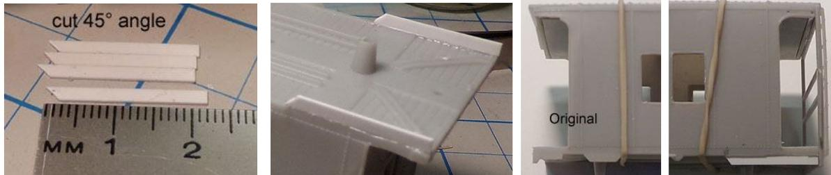
7. Next you will want to install the curved grab irons on the sides and the "L" shape grab irons on both sides of the rear door. (Below right photo) Detail Associates L Shape Grab Irons template included. The end railing was test fitted earlier. You might want to install them after everything is painted. Trying to paint the grab irons yellow afterwards may be difficult. Next add the 4 steps.
